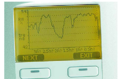
The display can be used to trace measurement trends back for up to a year.
