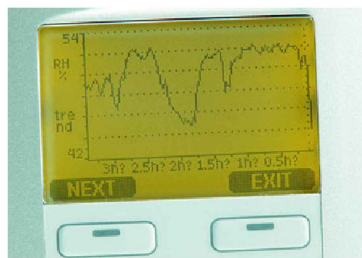
The display can be used to trace measurement trends back for up to a year.
